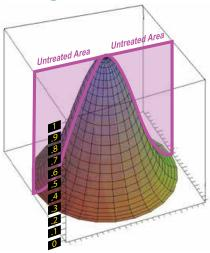
The picture above shows the typical electromagnetic field for one of the flat coils placed inside a therapy mattress. As you move away from the coil the magnetic field diminishes. This means that although the pulsing field will completely penetrate the body, some "dead" areas will occur (as shown in the purple areas of the picture).
